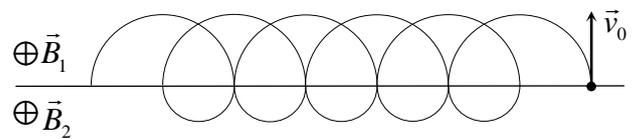
$$\Delta x = 2(R_1 - R_2) = \frac{2mv_0(B_2 - B_1)}{qB_1B_2}$$
